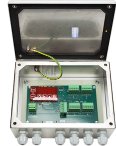
Optional stainless steel IP65 version (cover is not transparent)
